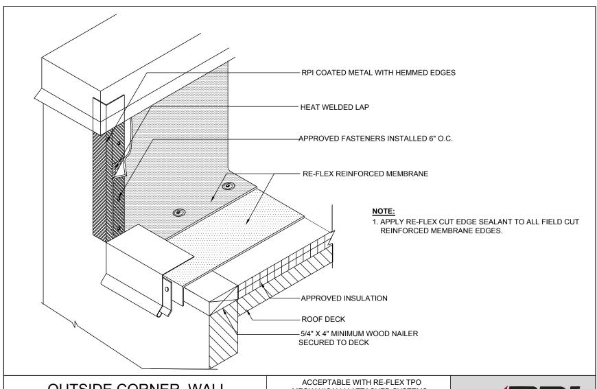
**OUTSIDE CORNER WALL** FLASHING WITH COATED METAL **DETAIL**
