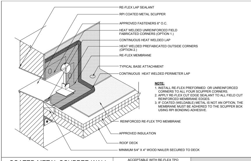
COATED METAL SCUPPER WALL FLASHING DETAIL
