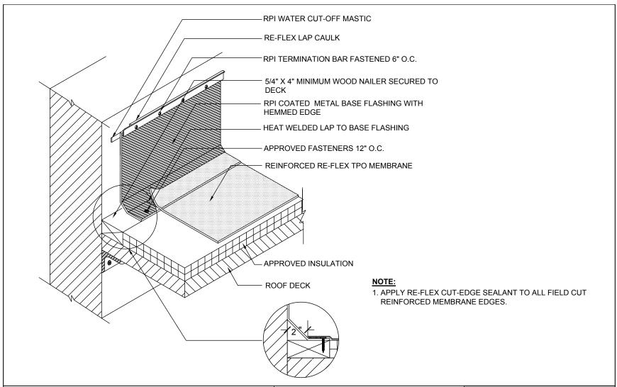
COATED METAL WALL FLASHING DETAIL
