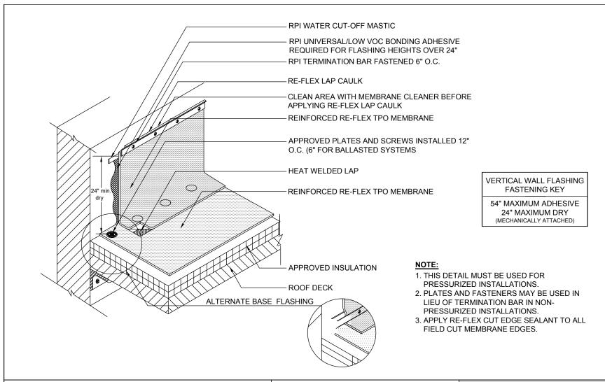
RE-FLEX TPO ADHERED WALL/CURB FLASHING WITH TERMINATION BAR DETAIL ACCEPTABLE WITH RE-FLEX TPO MECHANICALLY ATTACHED SYSTEMS
