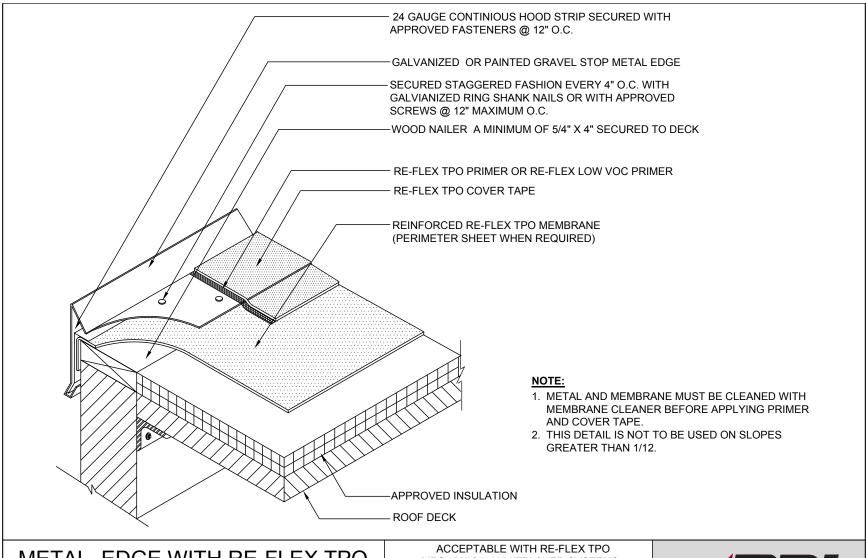
METAL EDGE WITH RE-FLEX TPO **COVER TAPE DETAIL**
