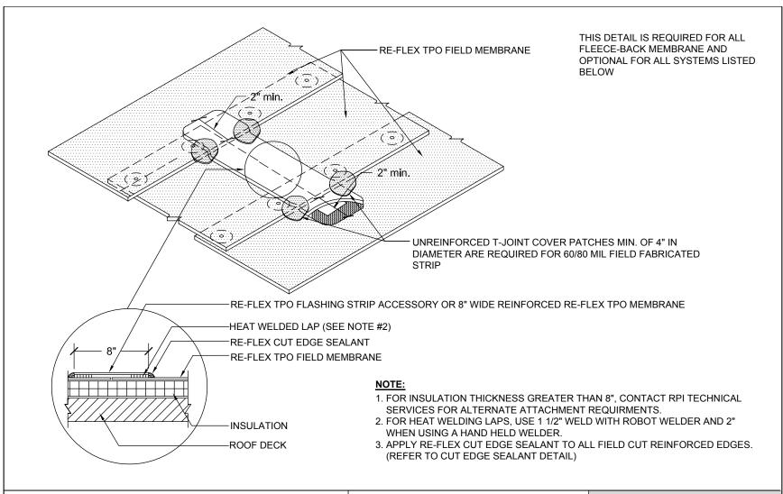
RE-FLEX TPO COVER STRIP HEAT WELD END LAP DETAIL
